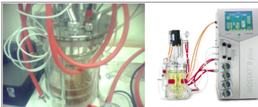
Figure 17. The Fermentor Biostat B-Plus, linked to a computer controlled interface for automatic monitoring and adjustment of stirring rate, temperature, pH and O_2 -supply [36] .
